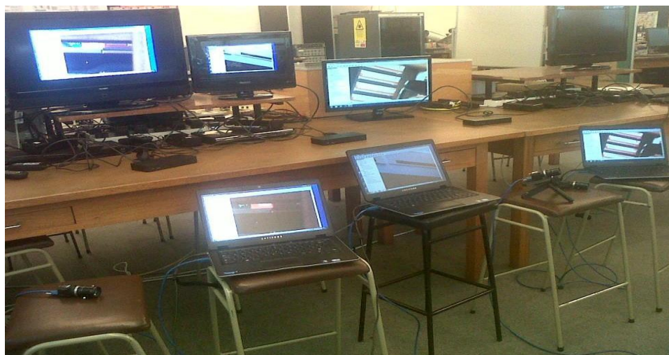
Fig 3: 4K UHD streaming over multi-channel 802.11ad
